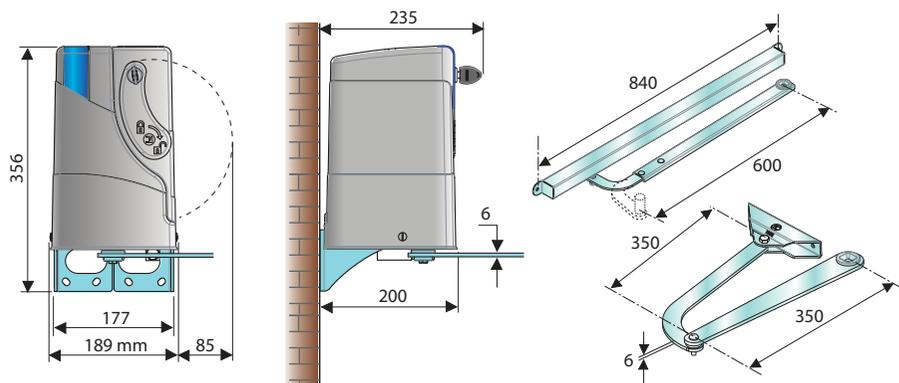
**BART 350** is an electromechanical gate system fitted with an arm, either cranked or straight (both made of zinc-coated steel) for residential swinging gates, semi-intensive use, designed for gate post mounting.
